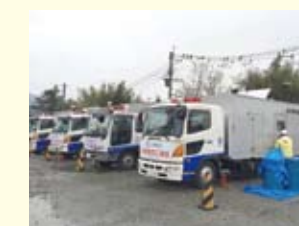
Power delivery to hospitals, etc. by four high voltage power generation vehicles
