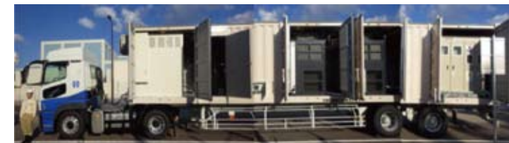
Installation of transportable nitrogen supply device
