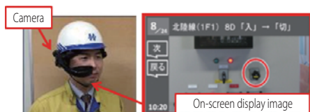
Example of remote assistance with a wearable camera and monitor
