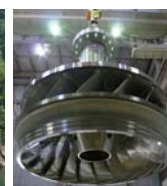
Hydraulic turbine runner at Arimine No. 2 Power Station
